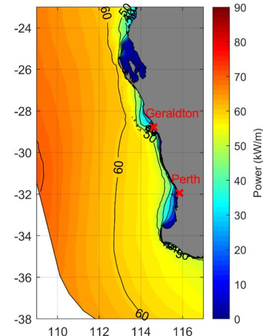
Left: Refraction of centroid wave parameters using MIKE21 SW with 1 km mesh at coast
